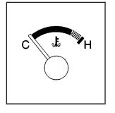
This gage shows the engine coolant temperature. If the gage pointer moves to the H (red) side, your engine is too hot.
